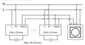
Set Dip switch to broadcast. All devices, max 26, would be controlled as a group.
