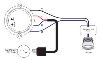
This phase dimmer adopts trailing edge dimming (reverse phase control), please make sure the connected loads support reverse phase control. Please refer to the user manual of the load or consult the supplier of the load.
