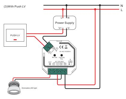
This phase dimmer adopts trailing edge dimming (reverse phase control), please make sure the connected loads support reverse phase control. Please refer to the user manual of the load or consult the supplier of the load.
