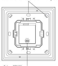
Battery: CR2430 Before the first use, please open the battery cover and remove the protective film
